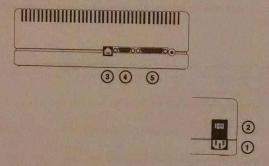
Figure 2 Connector Locations on the 213AE
