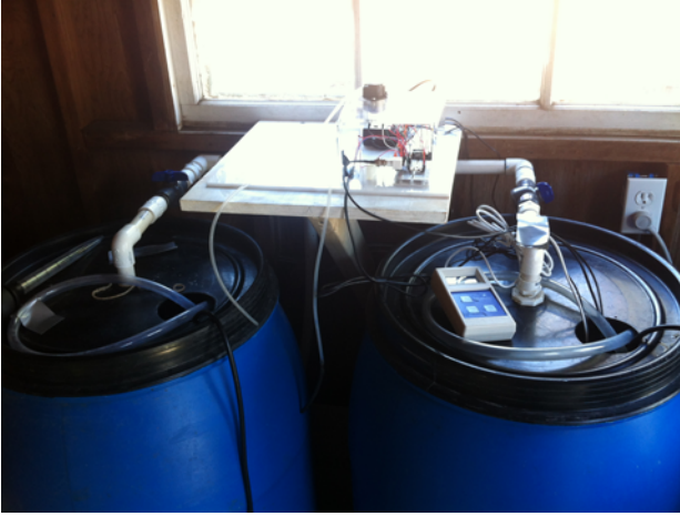
Figure 3-3. Reactor module that generates a healthy biofilm for hydroponic systems.
